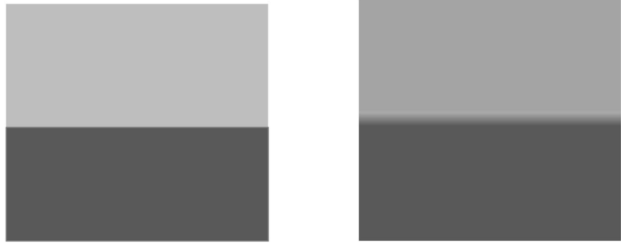
Fig. 1 The abrupt (left) and diffused (right) interfaces between two media in a contact
