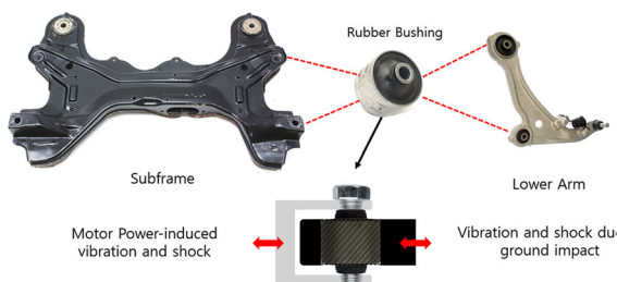
Fig. 2 Schematic of an automobile suspension system and the rubber bushing which connects the sub frame to the lower control arms
