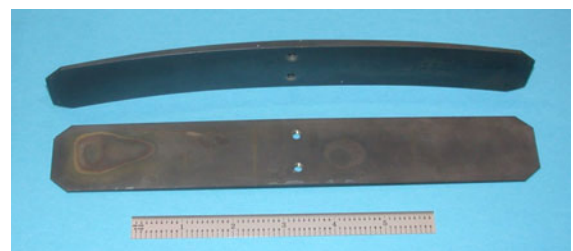
Fig. 20 Nitinol-60 flexure actuators used for flight test before (bottom) and after (top) heat treat processing
