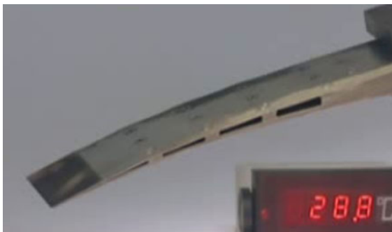
Fig. 26 Sub element of SMA bender structure
