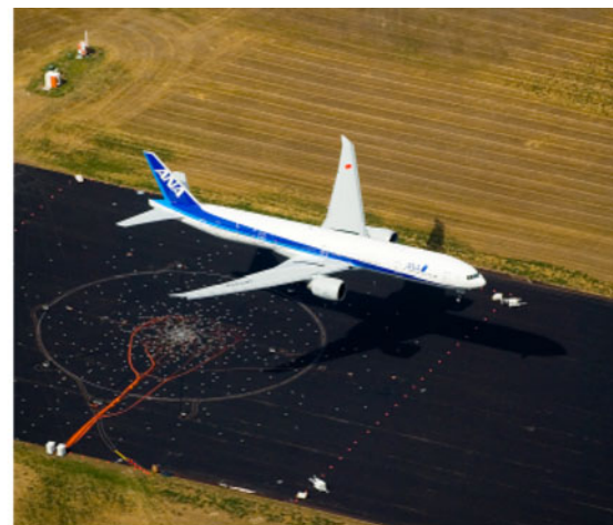
Fig. 18 Flight test of VGC mounted on GE90-115B engine on a ANA 777-300ER as part of the Quiet Technology Demonstrator 2 program
