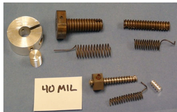
Fig. 11 Examples of the mandrels and collets discussed in the fabrication section of the high temperature SMA actuator case study, as well as some of the springs
