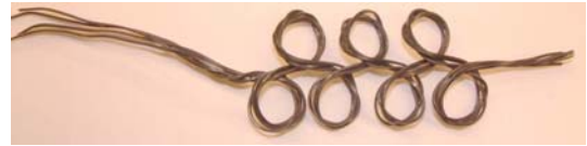
Fig. 1 SMA artificial muscle
