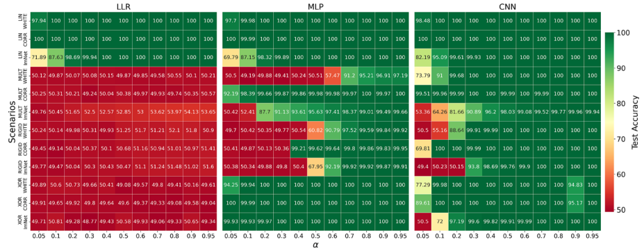
Fig. 4 Average test accuracy over 10 model trainings for each problem scenario and model architecture, for a fixed range of signal-to-noise ratios (SNRs). As expected, the Linear Logistic Regression (LLR) model cannot perform above chance level for non-linear scenarios. The Convolutional Neural Network (CNN) outperforms the Multi-Layer Perceptron (MLP) for the RIGID (translations and rotations of tetrominoes) scenarios as expected, perhaps due to the invariance under these properties for this architecture
