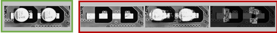
Fig. 8 (Color online) Zoomed area ( \approx X10 ) of a normal product image (left-green-framed 1st image) and an abnormal product image (right-red-framed image). One can see in the abnormal image that the input (2nd image) presents a pretty large defect (absence components), reconstructed with artefacts (3rd image) but still well patched (4th image)
