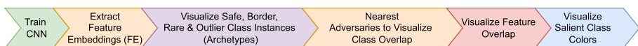
Fig. 1 Outline of the main components of our IML framework for imbalanced learning
