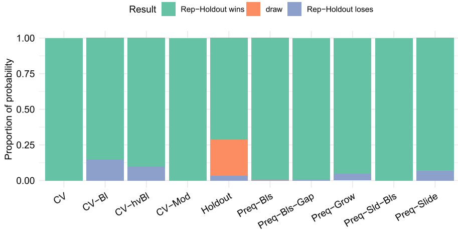
Fig. 14 Proportion of probability of the outcome when comparing the performance estimation ability of the respective estimation method with the Rep-Holdout method with non-stationary real-world time series. The probabilities are computed using the Bayes signed-rank test using the RBR learning method
