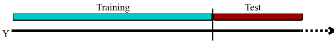
Fig. 1 Simple out-of-sample procedure: an initial part of the available observations are used for fitting a predictive model. The last part of the data is held out, where the predictive model is tested
