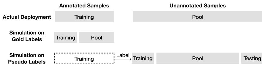
Fig. 3 Simulation on pseudo labels compares active learning methods on a large pool with noisy labels. In addition to the original validation and testing set, we also use a testing set with pseudo labels for evaluation
