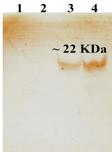
Fig. 5 The western blot results of human growth hormone protein. 1—The negative control sample (BL21 non-transformed bacterial extract), 2—hour 0 (before induction of hGH gene expression with IPTG), 3—2 h after induction of hGH gene expression with IPTG, 4—5 h after induction of hGH gene expression with IPTG. As expected recombinant human growth hormone protein has a molecular weight of about 22 kDa
