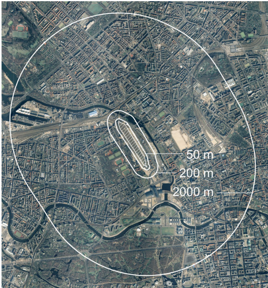
Fig. 2 Aerial image of an exemplary wasteland site ( shaded ) and three buffer zones (50, 200, and 2,000 m) for which population density and degree of sealing were calculated (Orthophotomosaik Berlin, © GeoBasis-DE/SenStadtUm III, 2005)
