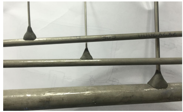
Fig. 3 Various test segments of stainless steel grade 316 with different diameters (2mm, 4mm and 5mm)
