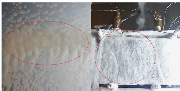
Fig. 6 Foam produced after release of the microemulsion inhibitor
