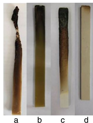
Fig. 1 Digital photographs of sample after UL-94 tests a sample 1; b sample 3; c sample 9; and d sample 10
