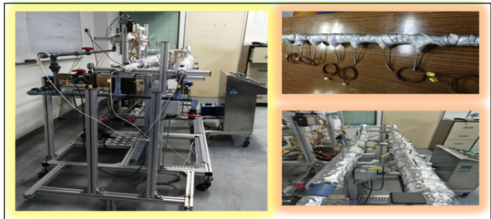
(b) Pictorial view of complete heat transfer test rig showing varying parts along with heat exchangers.
