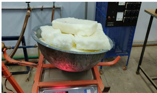
Fig. 2 Before melting and stirring operation the basic PCM
