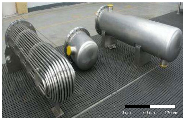
Fig. 1 A Typical shell and tube heat exchanger used in a chemical industry
