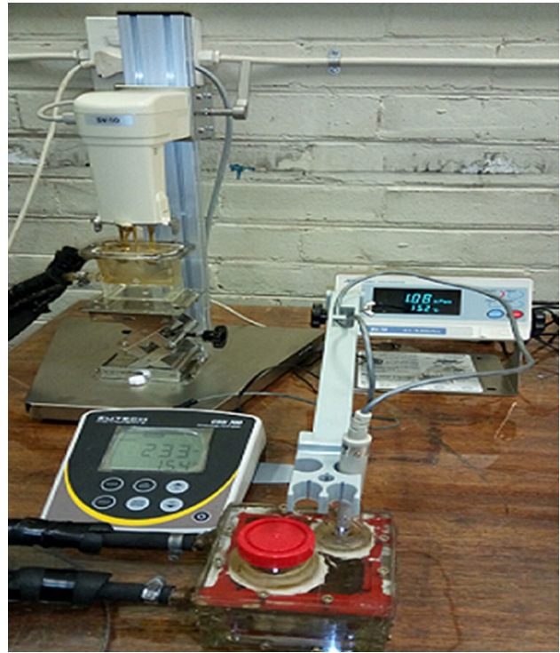
Fig. 1 Experimental set-up for viscosity and electrical conductivity
