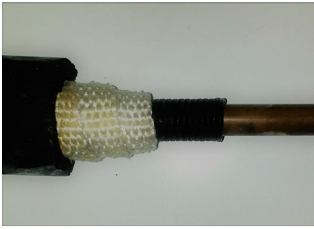
Fig. 3 Copper tube, element heater and glass wool insulation
