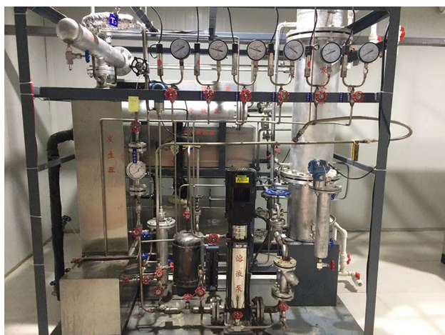
Fig. 21 Test rig for investigating the influence of TiO 2 nanoparticles on AARS [377]
