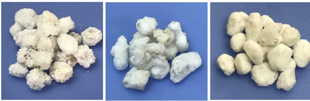
Fig. 3 Expanded perlite particles (left), EP filled with paraffin (middle), EP/PA coated by styrene (right)
