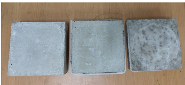
Fig. 9 Concrete blocks after thermal evaluation tests [ordinary concrete (left), surface-modified EP/PA (center), EP/PA composite (right)]
