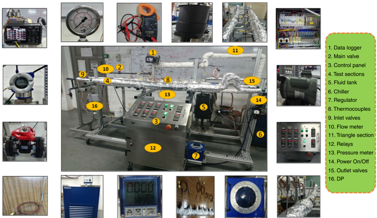
Fig. 5 Experimental setup with different parts for heat transfer measurements
