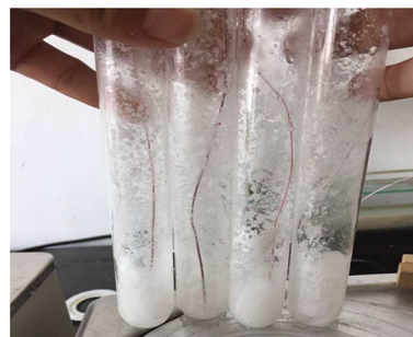
Fig. 8 Phase stratification of samples with 5 mass% of Na 2 B 4 O 7 ·10H 2 O as nucleating agent and different amounts of CMC
