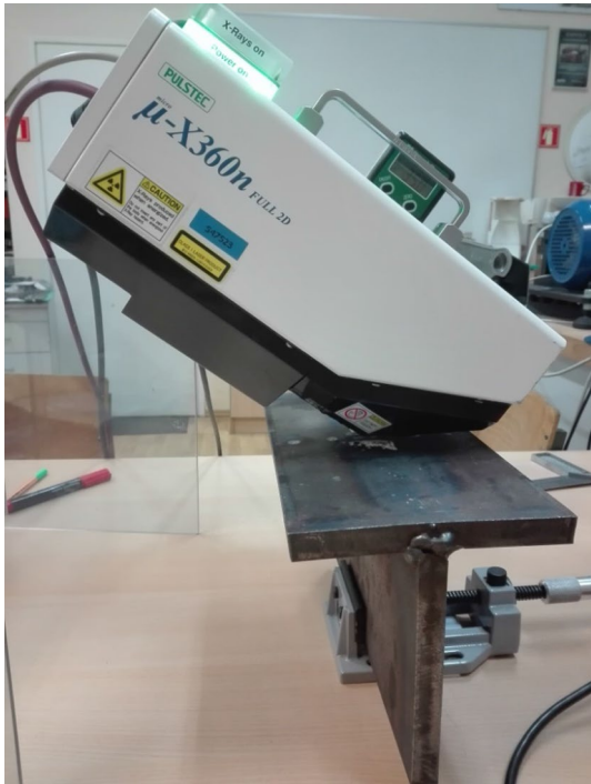
Fig. 5 Residual stress measurement using Pulstec \mu -X360 device
