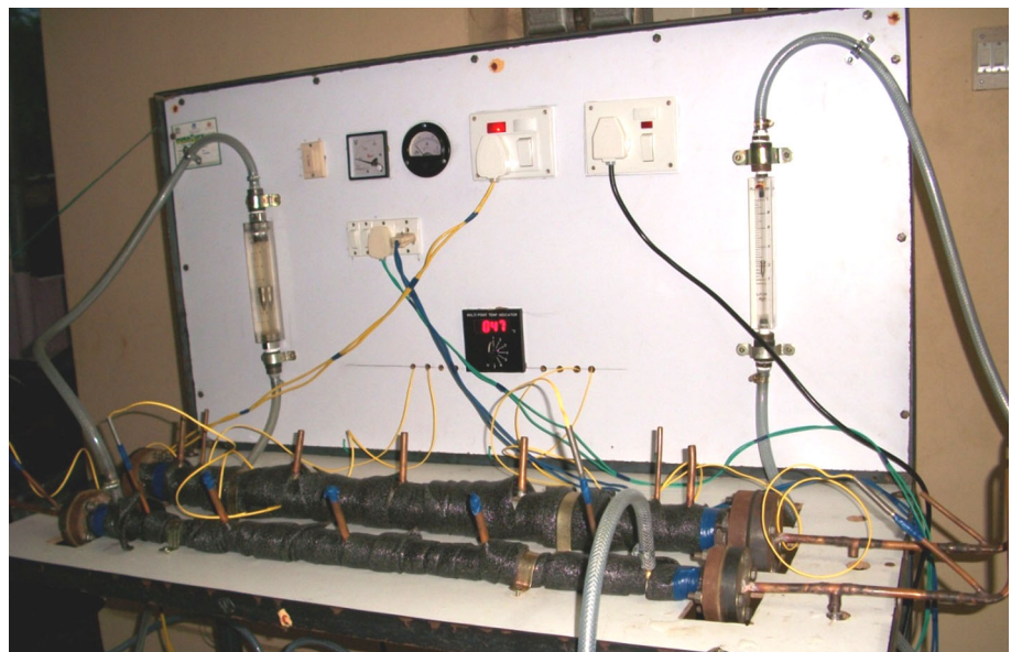
Fig. 1 Schematic diagram of double-pipe counter-flow heat exchanger
