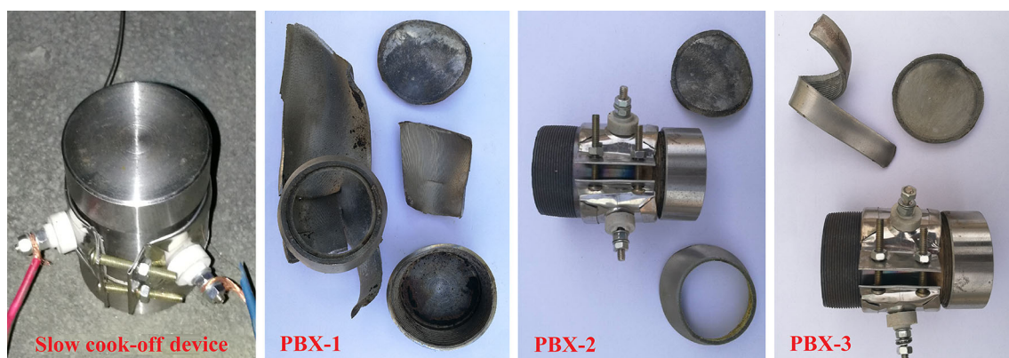
Fig. 8 Slow cook-off results of PBX-1, PBX-2 and PBX-3
