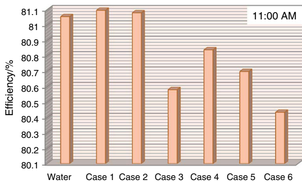
Fig. 41 Thermal efficiency of solar collector for different cases (adapted from the publication of Mahian O et al. [47] with the permission from ASME)
