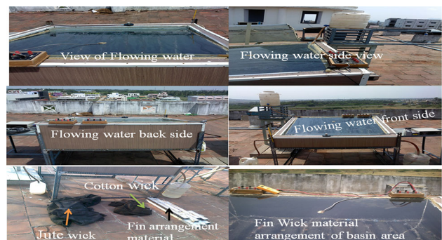
Fig. 4 Experimental trials of water flowing over the glass cover of a solar still with novel absorbing materials
