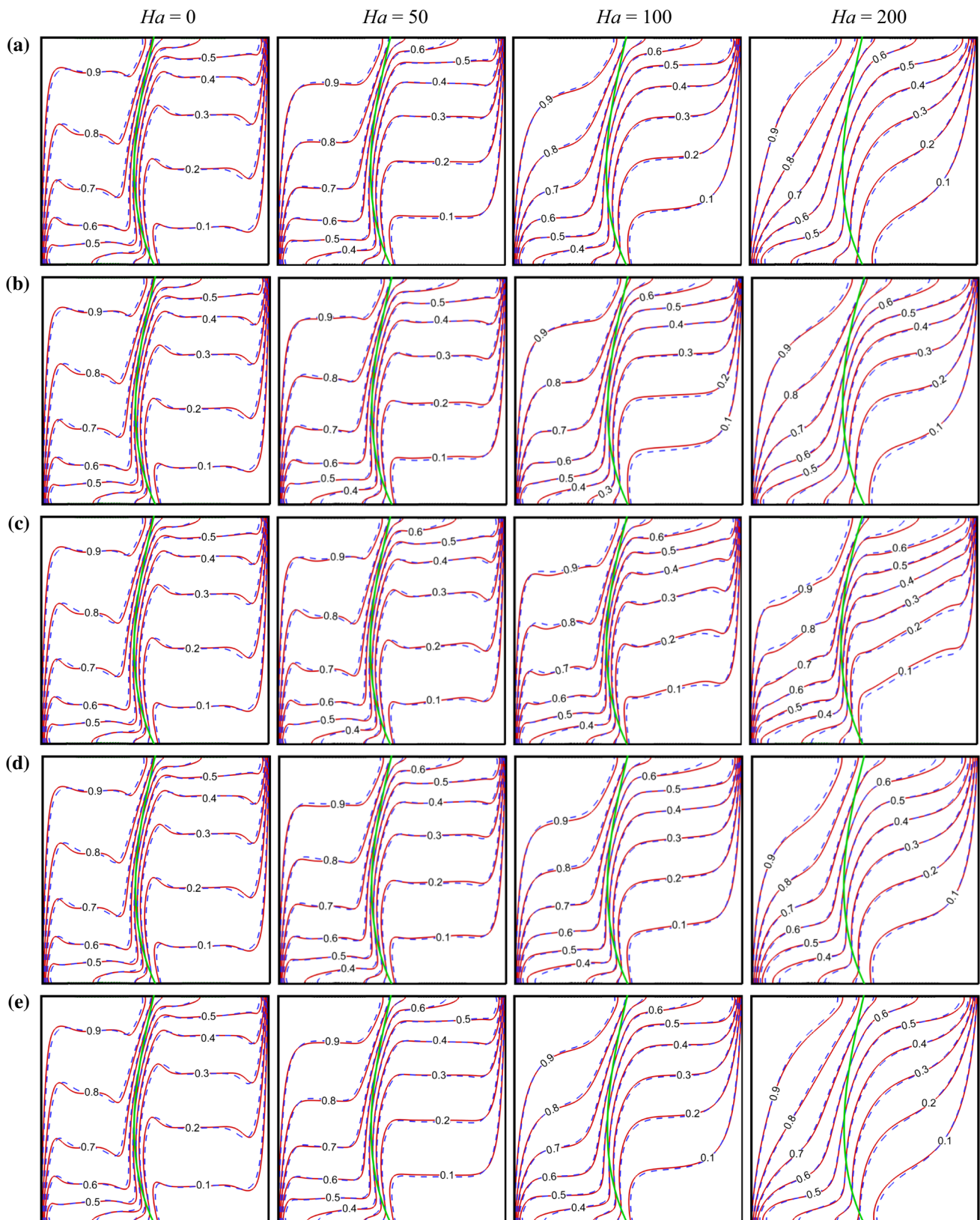
Fig. 14 The isotherms contours of the hybrid nanofluid (dashed lines) and the nanofluid with Al_2O_3 nanoparticles (solid lines) for different values of Ha in a \gamma = 0 , b \gamma = 45 , c \gamma = 90 , d \gamma = 135 and e \gamma = 180 for Ra = 10^7 and \phi_{hmf} = \phi_{Al_2O_3} = 2\%
