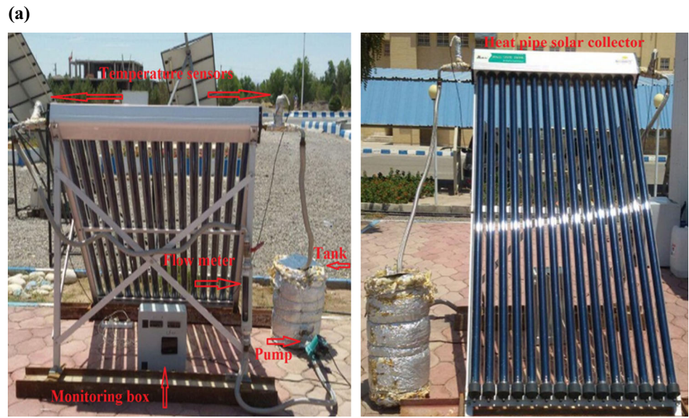
Fig. 1 Setup of the system at solar site of Vali-e-Asr university of Rafsanjan; a experimental setup, b simplified closed-loop system
