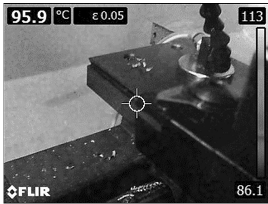
Fig. 7 Cutting tool temperature measurement
