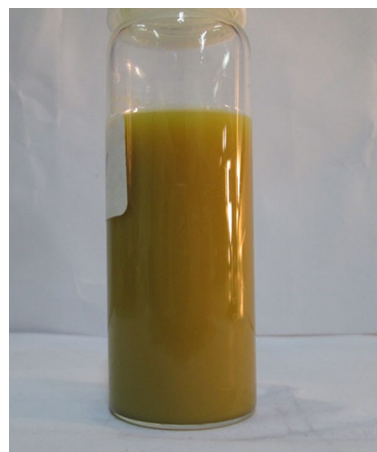
Fig. 6 The as-prepared Cu/CD suspension at 0.5 mass% after 1 month of stationary state
