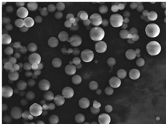
Fig. 1 SEM image of DMN-co-GMA copolymer
