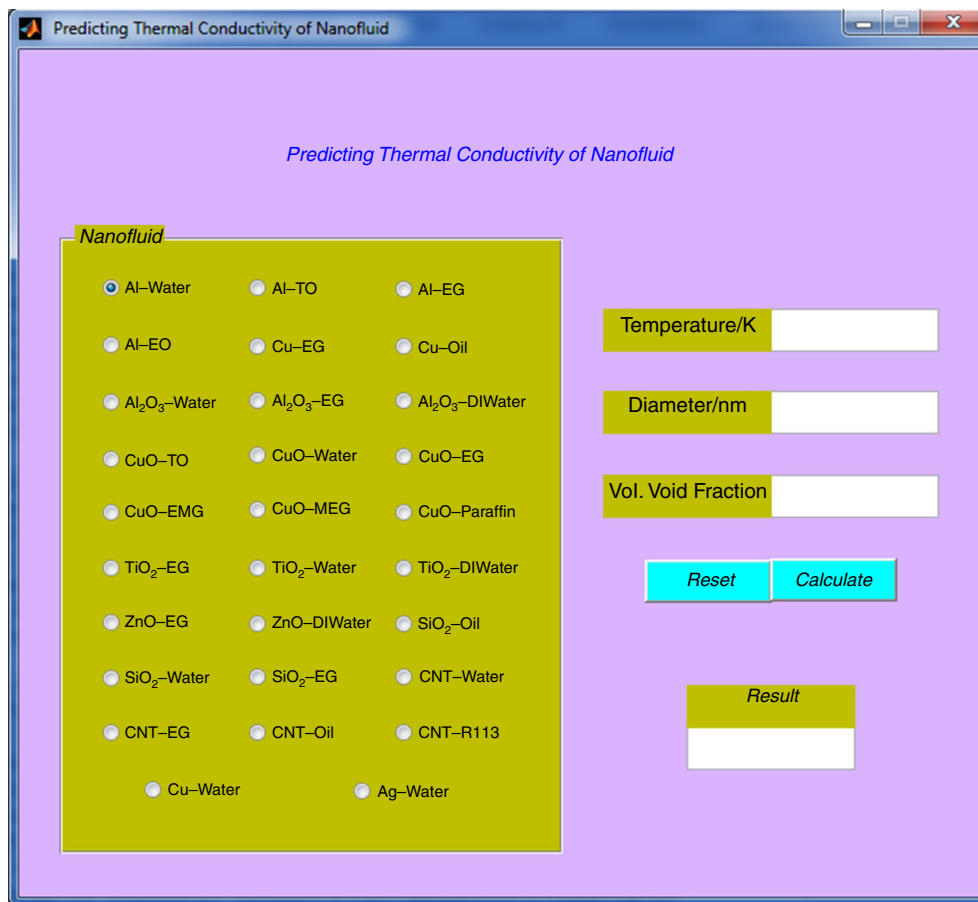
Fig. 15 GUI version of developed model for estimation of thermal conductivity of nanofluid
