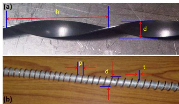
Fig. 8 a Twisted tape insert, b wire coil insert reprinted from Naik et al. [67] with permission from Elsevier
