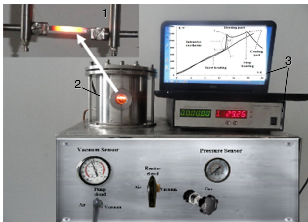
Fig. 1 Overall view of the HSTS-2 experimental setup: 1—Foil heater with reactive mixture and thermocouple. 2—Reaction chamber. 3—PC-assisted controller
