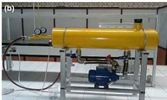
Fig. 2 a Scheme of laboratory system. b Laboratory-developed indirect heater
