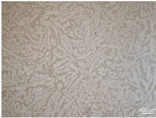
Fig. 1 Microstructure of the solution annealed material
