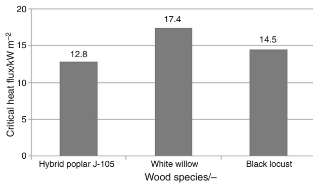
Fig. 4 Comparison of critical heat flux of hybrid poplar, white willow and black locust
