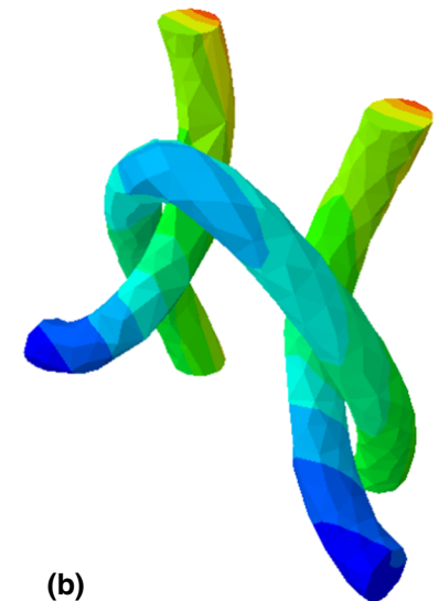
Fig. 10 Contours a heat flux and b temperature contour of plain weft knitted fabric unit cell
