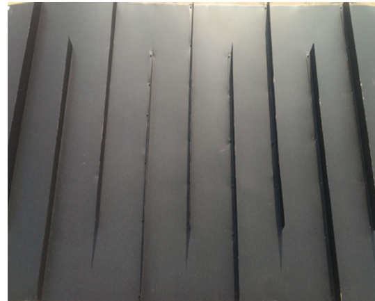
Fig. 1 Nanostructured and baffle-arranged absorber
