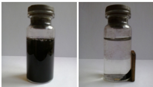
Fig. 5 Photograph of magnetic separation of rambutan-like \text{MnCo}_2\text{O}_4 obtained at 400^\circ\text{C} from the aqueous solution with a permanent magnet
