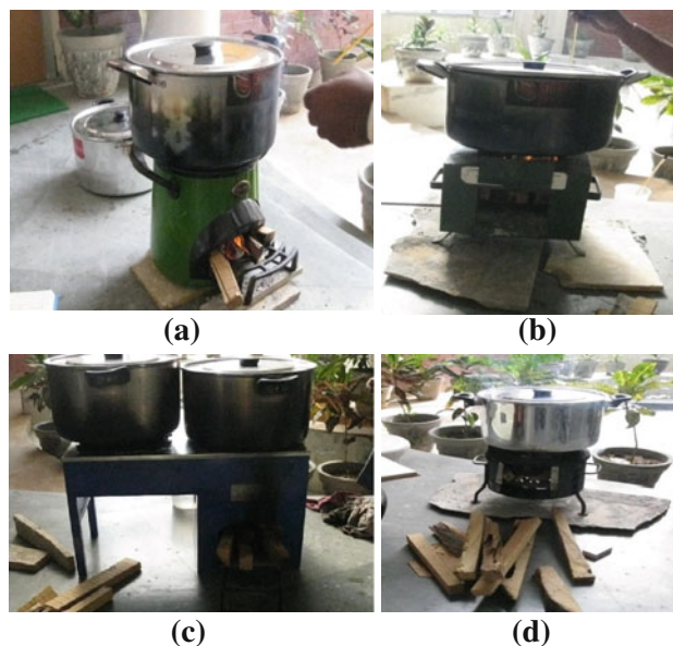
Fig. 1 a Envirofit model. b Harsha model. c Mangla model. d Vikram model. Photographic view of various cook stove models during experimental study
