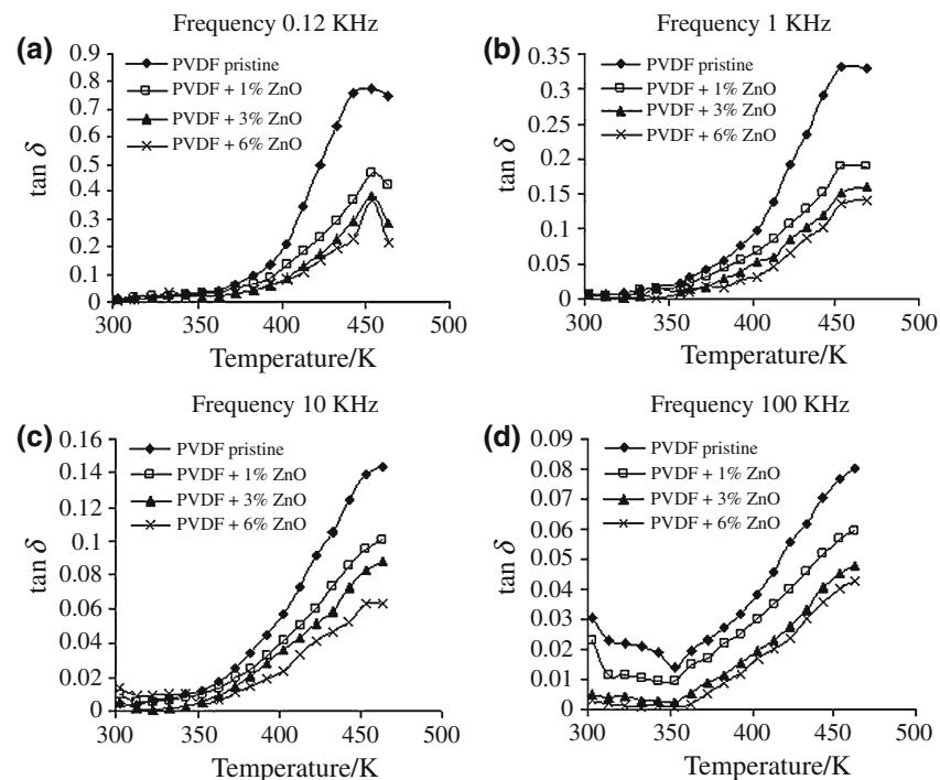
**Fig. 7** Tangential loss versus Log frequency plots of PVDF pristine and PVDF + ZnO nanocomposite samples at temperatures **a** 303 K, **b** 353 K, **c** 403 K, and **d** 463 K with different mass/% of ZnO
