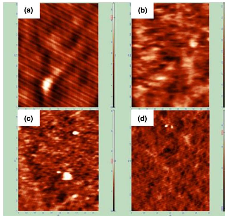
**Fig. 3** AFM-3D topographic image of **a** PVDF pristine, **b** PVDF + 1 mass/% ZnO nanocomposite, **c** PVDF + 3 mass/% ZnO nanocomposite, and **d** PVDF + 6 mass/% ZnO nanocomposite samples
