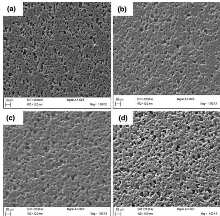
**Fig. 2** AFM-2D topographic image of **a** PVDF pristine, **b** PVDF + 1 mass/% ZnO nanocomposite, **c** PVDF + 3 mass/% ZnO nanocomposite, and **d** PVDF + 6 mass/% ZnO nanocomposite samples
