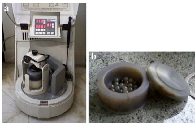
Fig. 1 a Ball mill set (Satellite mill). b Agate container and balls used in milling
