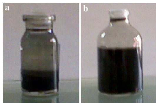
Fig. 2 Paraffin suspensions: a without oleic acid and occur settling and b with oleic acid and stability of suspension
