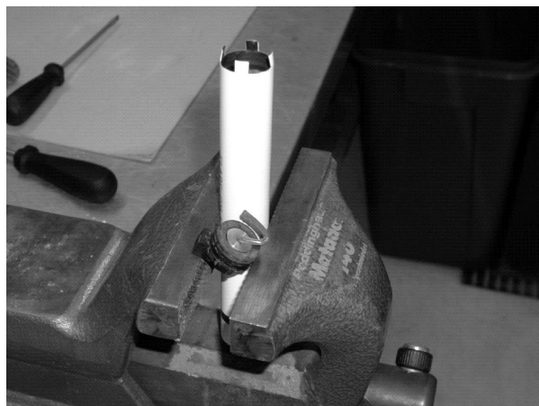
Fig. 2 End plug with igniter cord removed from (end plug not shown) the top of the tracer
