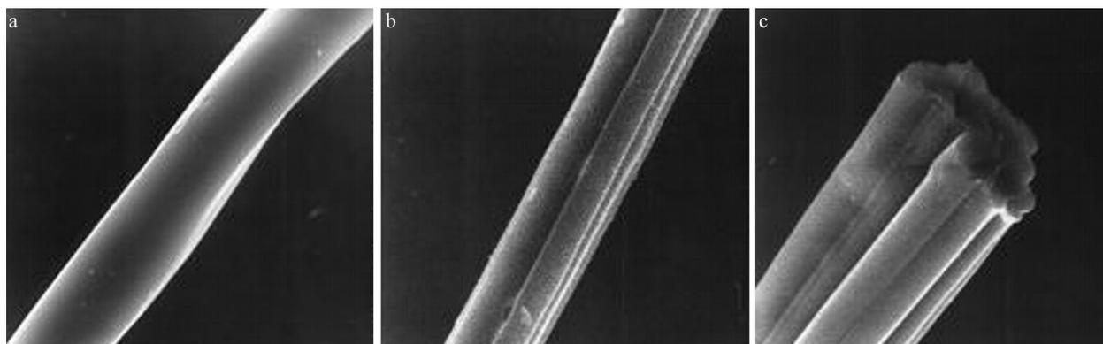
Fig. 6 SEM micrographs corresponding to fiber: a – lyocell, b – modal and c – viscose
