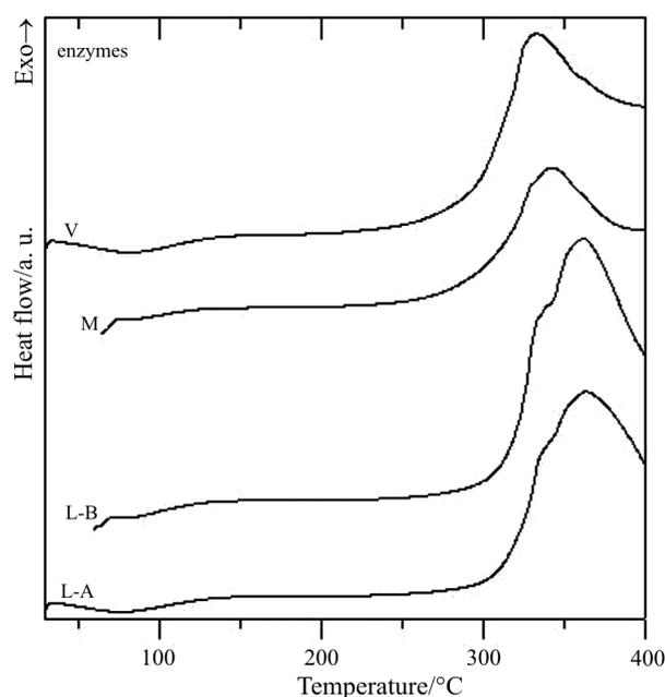
**Fig. 1** DSC scans of textile fibers with enzymatic treatment: L-A – lyocell, L-B – fibrillated lyocell, M – modal and V – viscose
