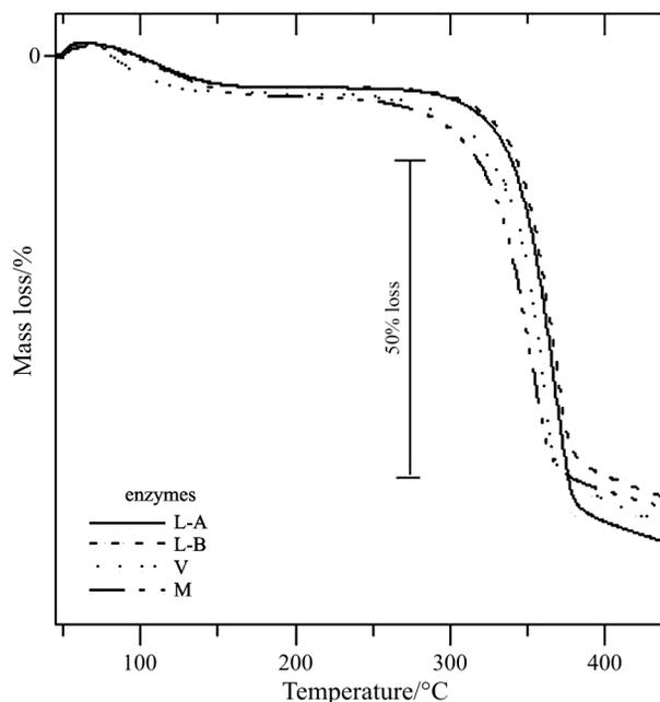
**Fig. 3** TG scans of textile fibers with enzymatic treatment: L-A – lyocell, L-B – fibrillated lyocell, M – modal and V – viscose
