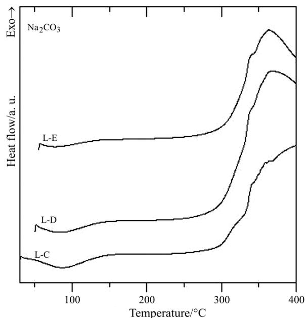
**Fig. 2** DSC scans of textile lyocell fibers after Na<sub>2</sub>CO<sub>3</sub> treatment: L-C, L-D – fibrillated and L-E – fibrillation and enzymatic treatment
