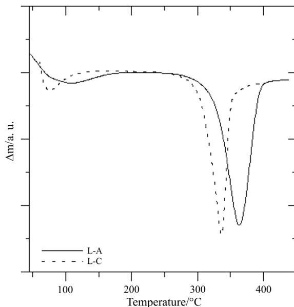
Fig. 5 DTG scans of textile lyocell fibers L-A and L-C
