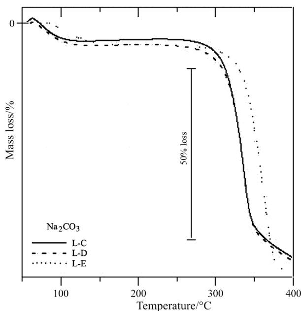
**Fig. 4** TG scans of textile lyocell fibers after Na<sub>2</sub>CO<sub>3</sub> treatment: L-C, L-D – fibrillated and L-E – fibrillation and enzymatic treatment
