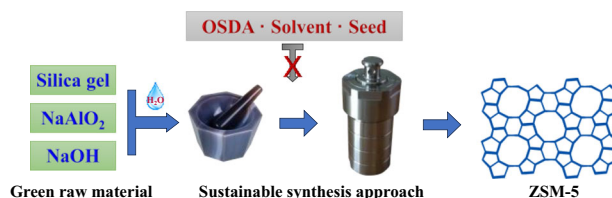
Fig. 1 Schematic representation for the sustainable synthesis of ZSM-5
