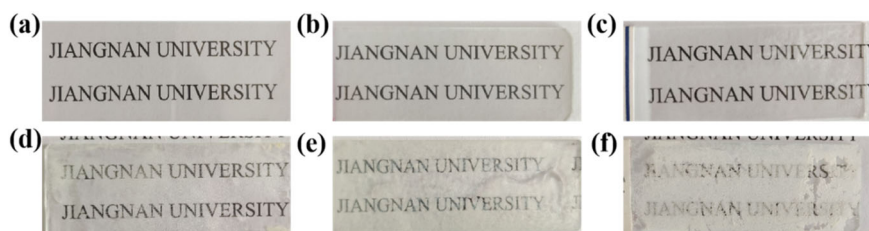
Fig. 7 Comparison of light transmittance between bare glass and coated glass (daytime lighting conditions): a was bare glass, and b–f were coated glasses. The dosage of silane coupling agent were (b) 0.1%, (c) 0.2%, (d) 0.3%, (e) 0.4%, and (f) 0.5%
