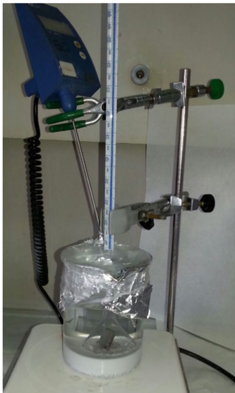
Fig. 1 Photography of dispositive for hydrogen evolution test
